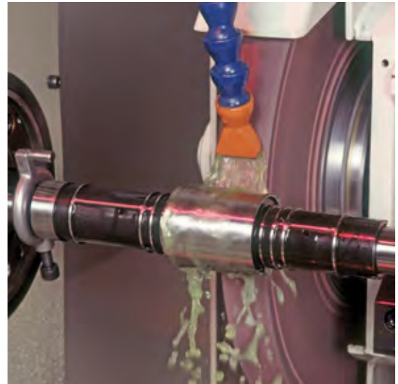
94AB BAS – Advanced grain technology used in Cylindrical and Centerless applications. This grain can be used to grind steels in either soft or hard state.
