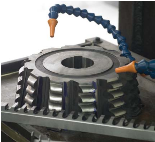
Straight oil lubricant with additive is applied to reduce friction and heat during the broaching operation.
