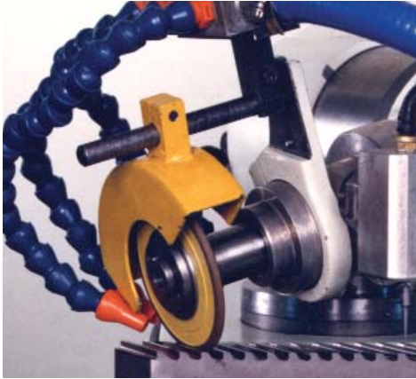
Aggressive cutting action required by grinding at high-material rates in creep-feed mode.
