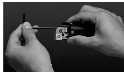
3. Tighten three screws to clamp the boring head.
