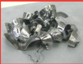
This picture indicates poor chip formation. Dull, torn, and undefined shape indicates poor cutting conditions.
