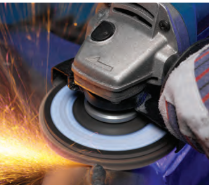
Blending and finishing a weld.
