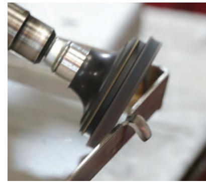
Edge chamfering a fabricated stainless component.
