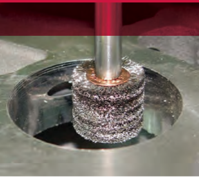
Deburring intersecting oil passages in an engine block.
