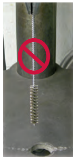
Incorrect Mounting in Chuck
