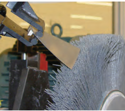
Deburring the tip of a turbine blade.
