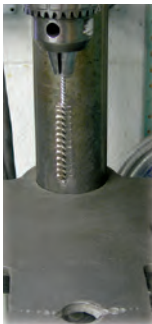
Correct Mounting in Chuck
