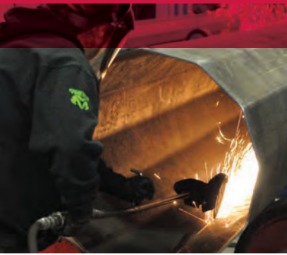
Weld removal with Tiger combo wheel.
