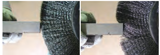
Correct Wire Tips Doing the Work
