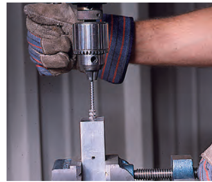
Crosshole deburring an aluminum manifold.
