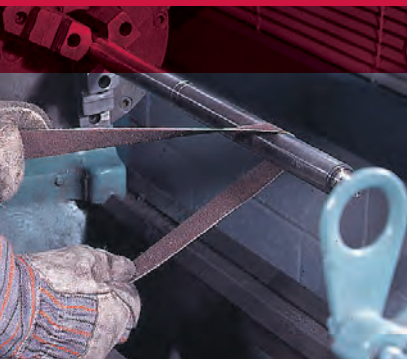
Polishing the O.D. of a part turning in a lathe.
