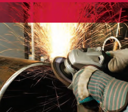
Beveling pipe on edge with a Tiger Paw flap disc.
