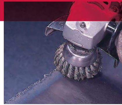
Removing slag from a flame-cut steel plate.
