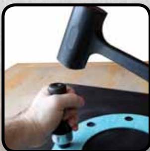
Remove centering pin and strike.
