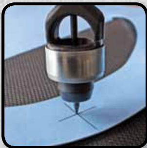
Position centering pin on target point.
