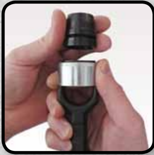
Mount cutting head into power punch handle.
