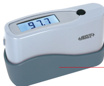
base with calibration block (included)
