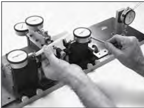
Inserting ceramic cylinder in gage to check squareness and parallelism of ends, longitudinal bow and out-of-roundness
