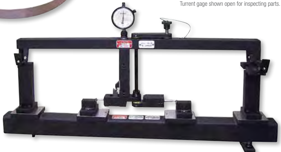
Turrent gage shown open for inspecting parts.
