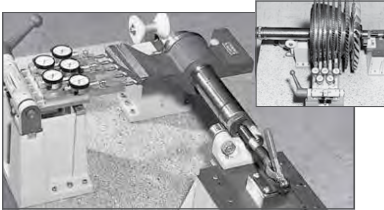
Inset: Rotor turns 360° on its axis to determine runout and radial deviation.
